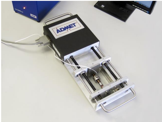
Figure 7: Admet eXpert 4000 with solution bath, recommended for durability testing of rubber components if experiment were to be repeated
